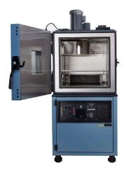
Left: For extreme testing, Russells offers a PCU equipped with  $\rm LN_2$  cooling for a wider cooling range and expedited temperature pull downs.
